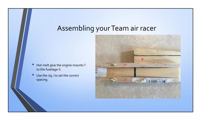
There is a jig to ensure the engine bearer is in the correct position so I suggest you use it.
