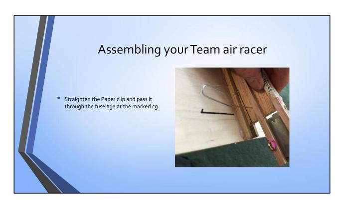
Straighten the Paper clip and pass it through the fuselage at the marked cg.
