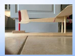
To ensure a stable airplane aerospace engineers will balance the airplane at about 20% of wing chord behind the leading edge.
