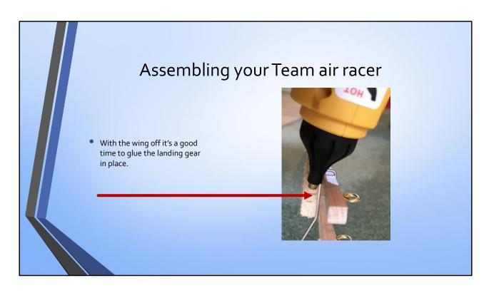
With the wing off it's a good time to glue the landing gear in place.
