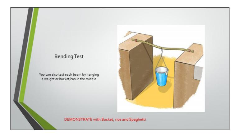
For Bending Test cut 20 cm long sections of Spaghetti.
