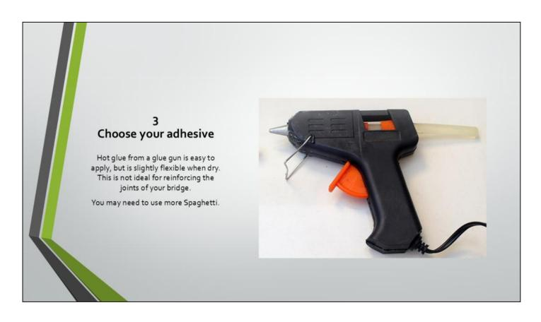
Hot glue from a glue gun is easy to apply, but is slightly flexible when dry. This is not ideal for reinforcing the joints of your bridge. You may need to use more Spaghetti.
