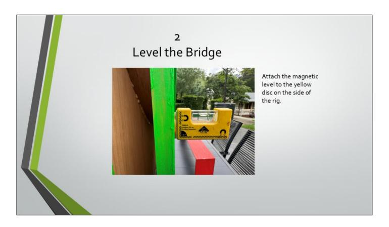
Level the bridge using the Stabilo magnetic level.
