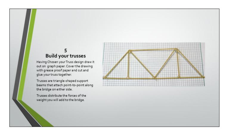
Having Chosen your Truss design draw it out on graph paper. Cover the drawing with grease proof paper and cut and glue your truss together.
